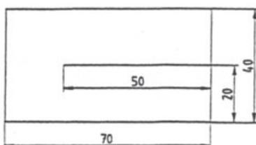
Double edged tear strength is tested according to DIN EN ISO 3377-2, IUP 8. A rectangular test specimen with a hole of specified shape is placed over the turned up ends of a pair of holders attached to the jaws of a testing machine.
