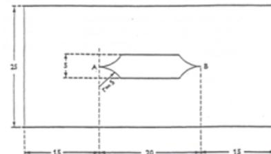
The highest force exerted during tearing of the test piece is recorded and expressed as “N”.
